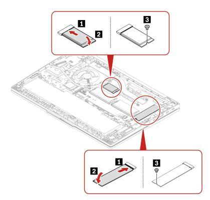
Step 2. Install the M.2 solid-state drive in reverse order.
