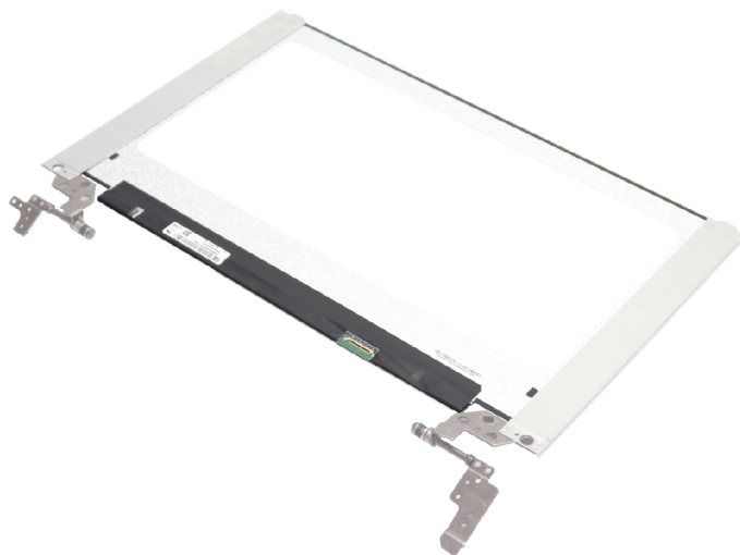
Figure 67. Remove the LCD assembly
