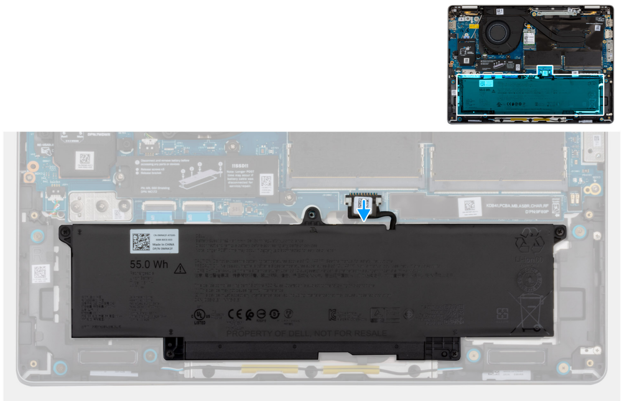
Figur 24. Disconnecting the battery cable
