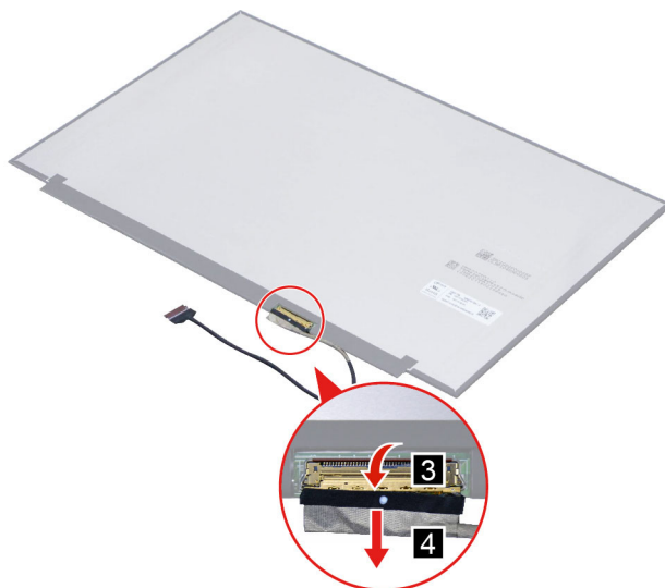
Figure 32. Remove the EDP cable
