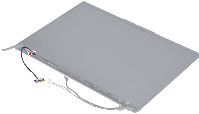
Figure 29. Release the EDP cable
