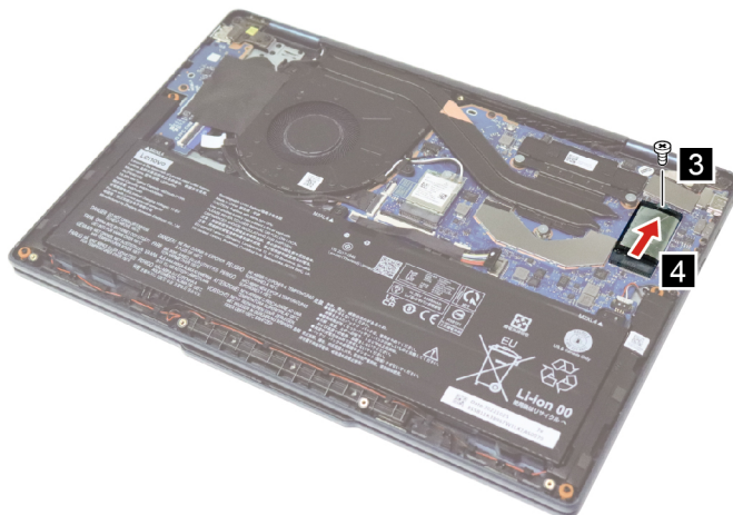
Figure 10. Remove the 2242 solid-state drive
