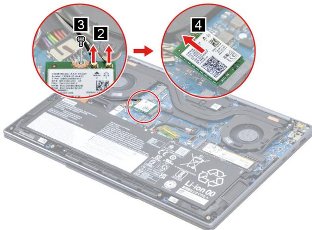
Figure 14. Remove the Wi-Fi card
