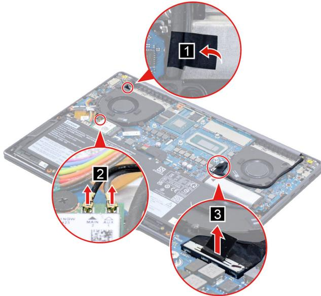
Figure 31. Disconnect the EDP cable and antenna cable
