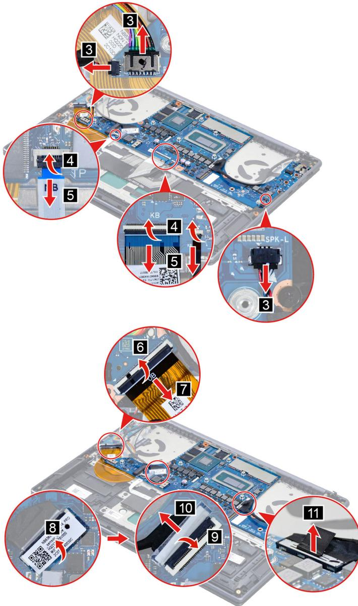
Figure 27. Disconnect cables connected to the system board
