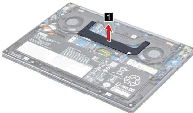
Figure 7. Remove the internal rubber
