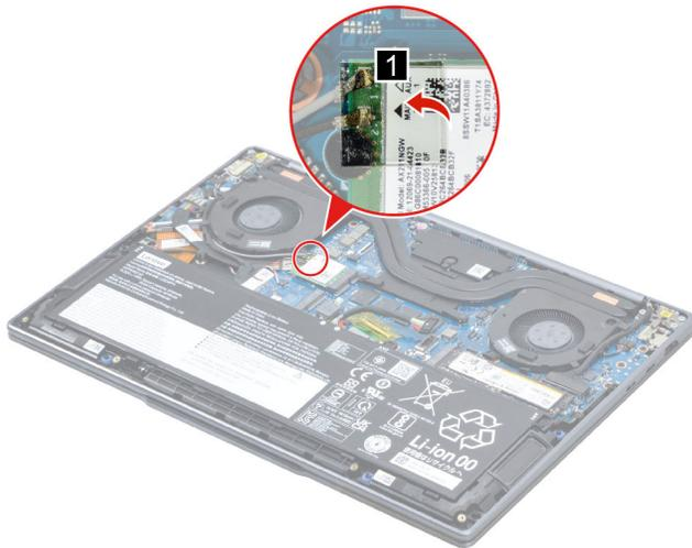
Figure 13. Remove the Wi-Fi card cover
