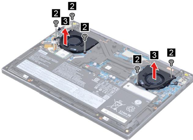
Figure 23. Remove five screws and remove the fan
