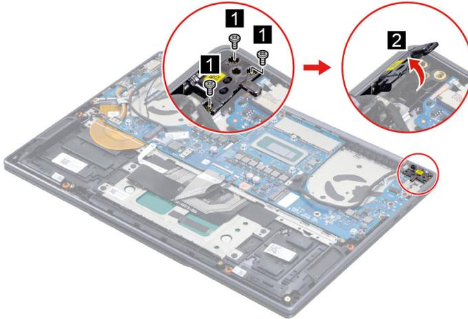
Figure 26. Remove three screws and open the hinge
