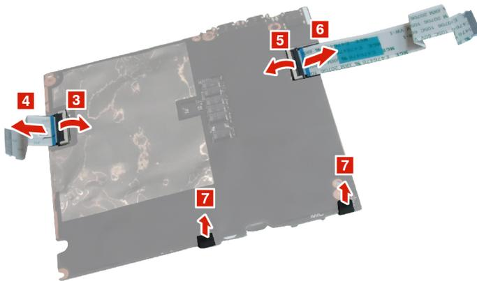
Figure 43. Disconnect the UB\_MB FFC and remove the microphone rubbers
