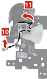
Figure 18. Remove the SWT PCB
