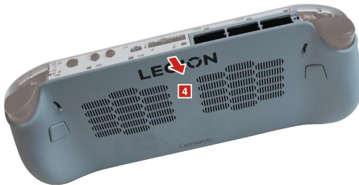
Figure 9. Remove the B cover
