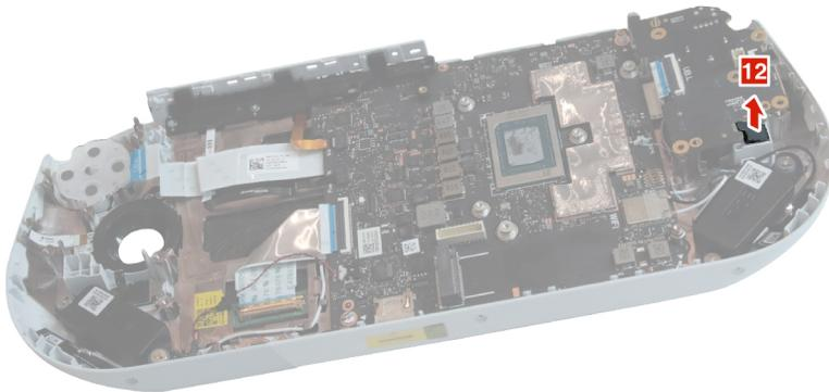
Figure 25. Remove the left motor
