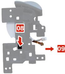
Figure 17. Remove the back key FPC
