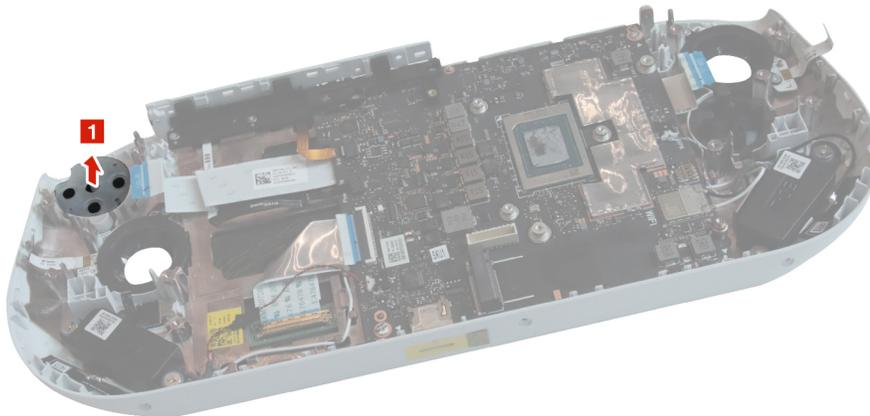
Figure 30. Remove the ABXY rubber
