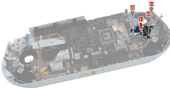
Figure 27. Remove screws and the D-pad board
