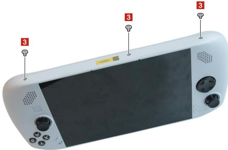
Figure 8. Remove screws at the bottom
