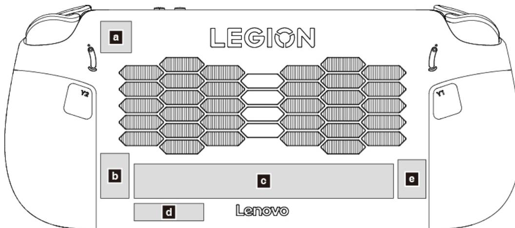
Figure 44. Label layout on the B cover
