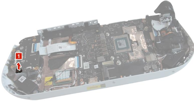
Figure 19. Remove the right motor
