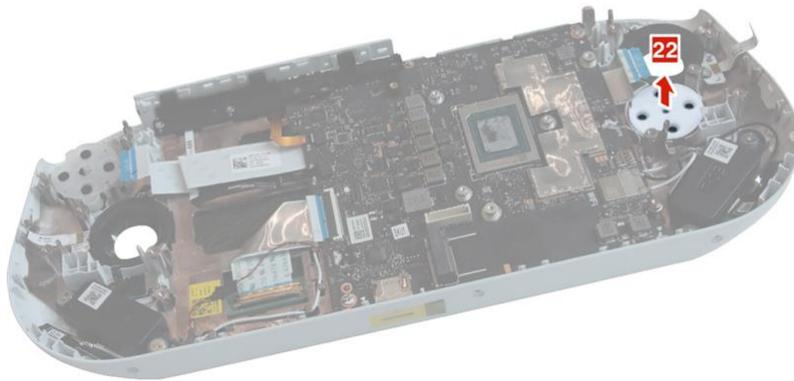
Figure 28. Remove the D-pad rubber
