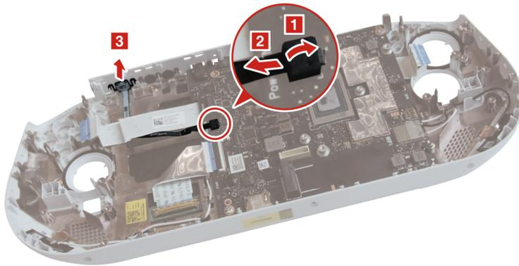
Figure 38. Disconnect the power button FPC and remove the power button
