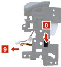
Figure 23. Remove the back key FPC
