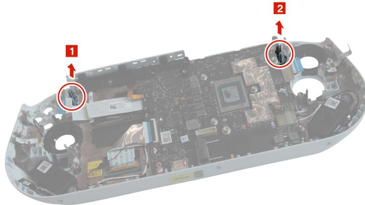
Figure 32. Remove the function buttons
