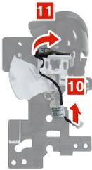
Figure 24. Remove the SWT PCB
