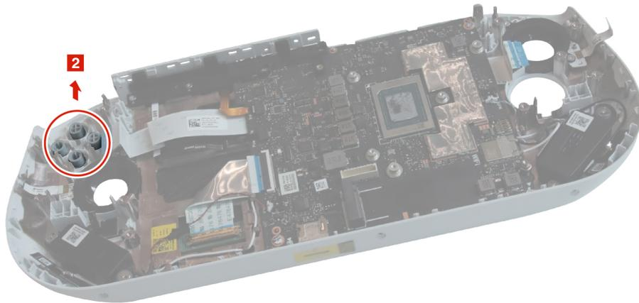
Figure 31. Remove the ABXY buttons
