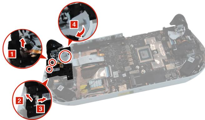
Figure 15. Disconnect the SWT PCB cable and disconnect the back key FPC
