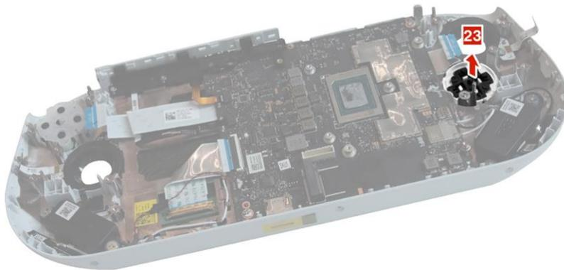
Figure 29. Remove the D-pad frame and D-pad button
