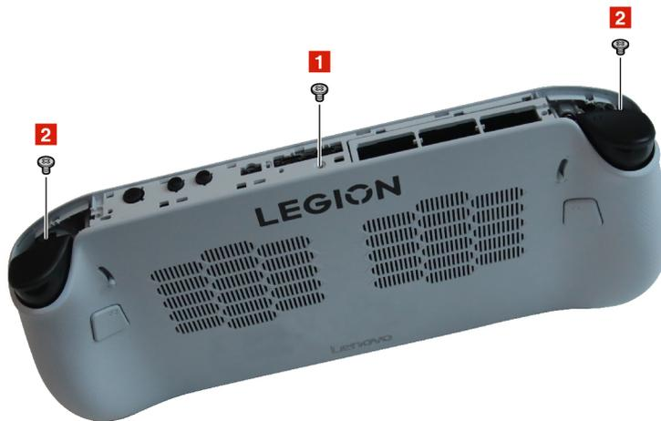
Figure 7. Remove screws at the top
