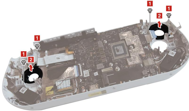
Figure 34. Remove screws and remove RGB lights
