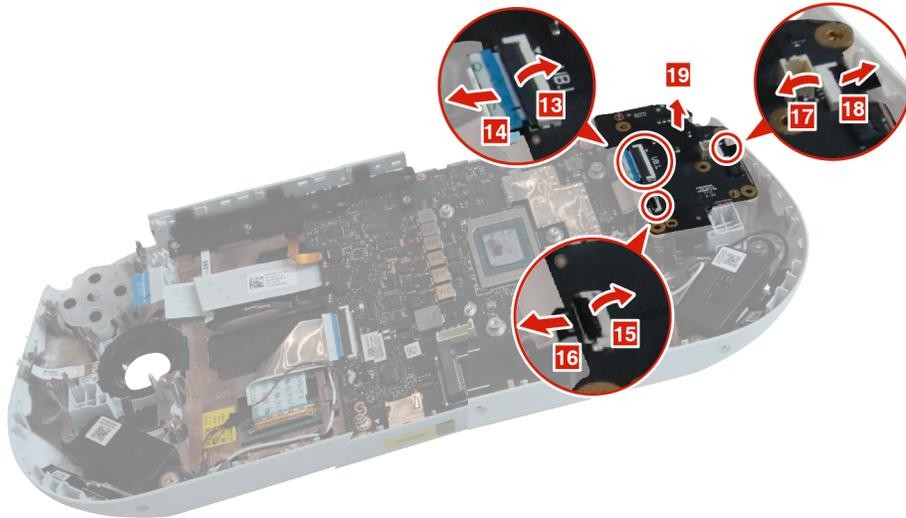
Figure 26. Disconnect the UB\_Ring FPC, disconnect the MB\_UB FFC, disconnect the D-pad board FFC, and remove the left board
