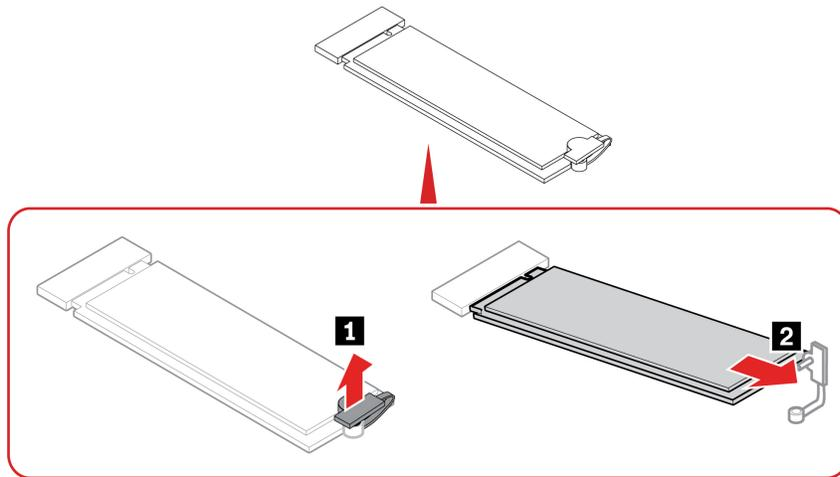
**Note:** Remove the film that covers the thermal pad (if any) when installing the M.2 solid-state drive.
