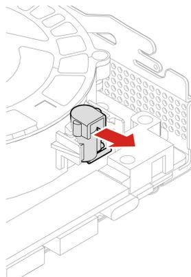
3. Disconnect the system fan cable from the system fan connector on the system board.
