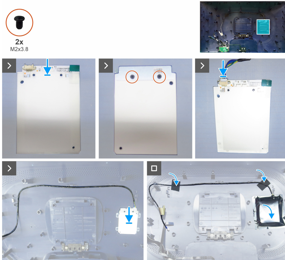
Figure 14. Installing the backlight module
