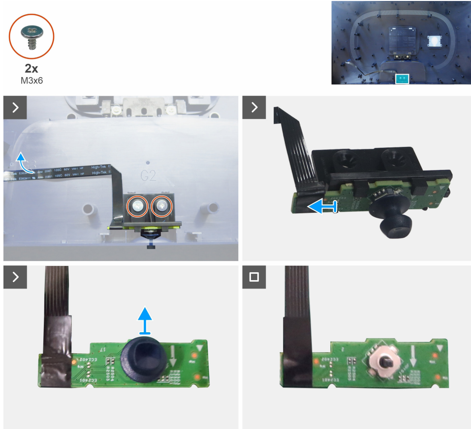
Figure 9. Removing the joystick board
