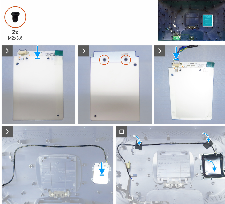
Figure 6. Installing the backlight module
