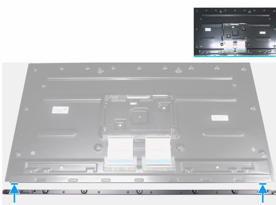
Figure 18. Installing the front trim
