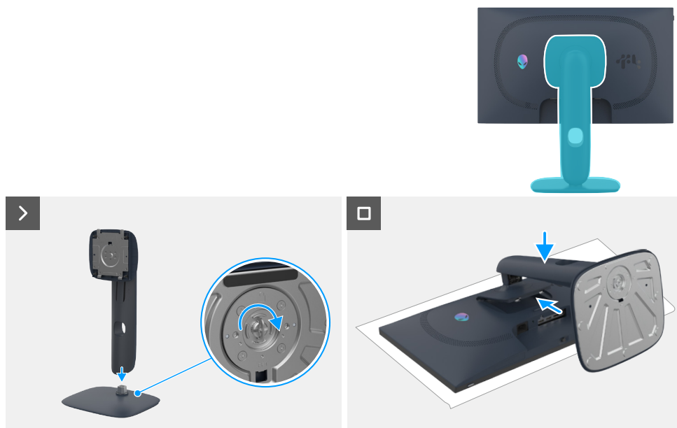
Figure 10. Installation du socle
