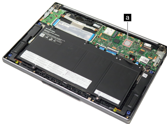
Figure 3. Area on the system board where thermal interface material is applied
