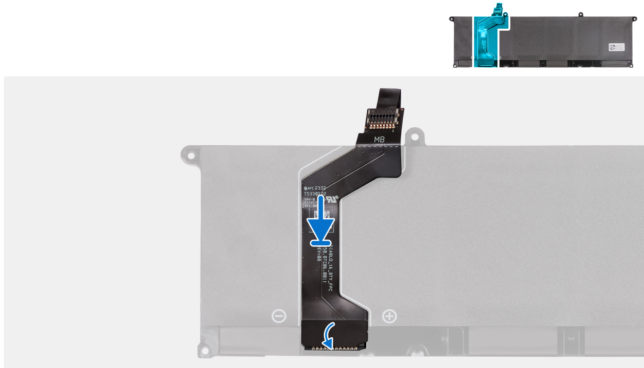
Figure 11. Installing the battery cable
