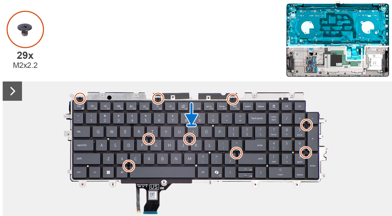
Figure 85. Installation du clavier
