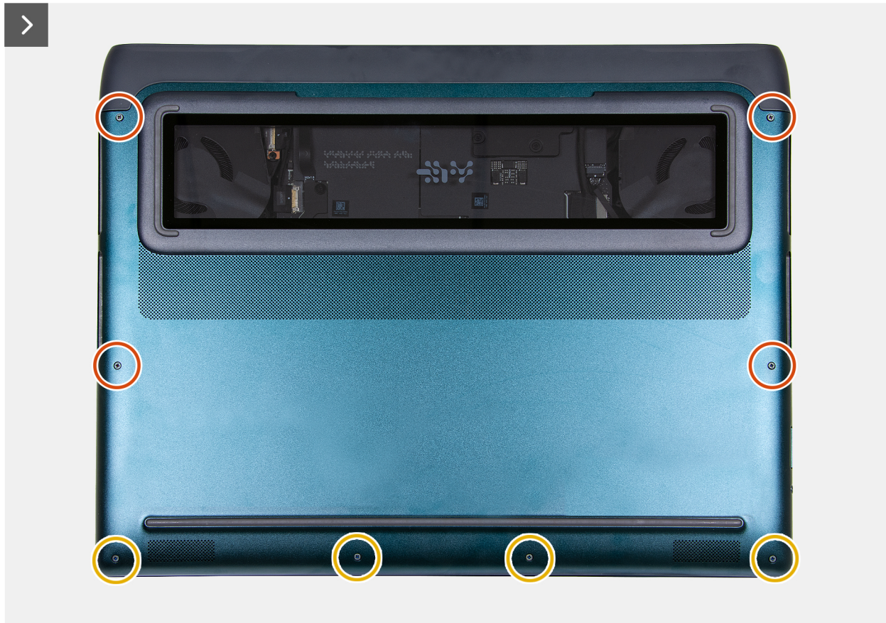
Figure 9. Removing the base cover screw
