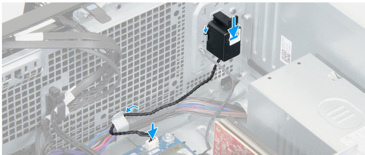
**Figura26. Instalar a coluna interna**
