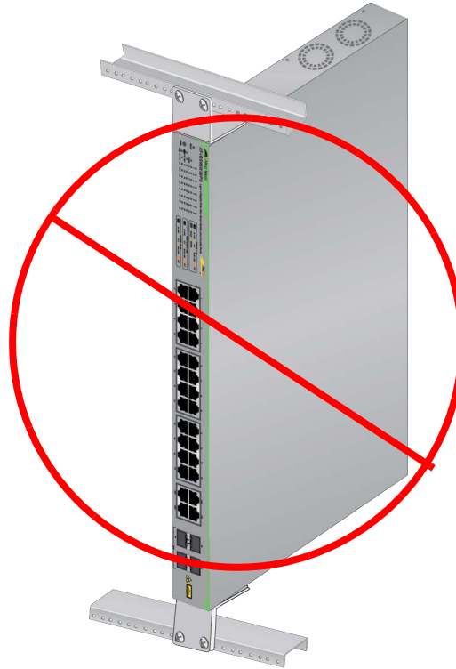
Figure 22. Switch in a Vertical Equipment Rack - Not Supported
