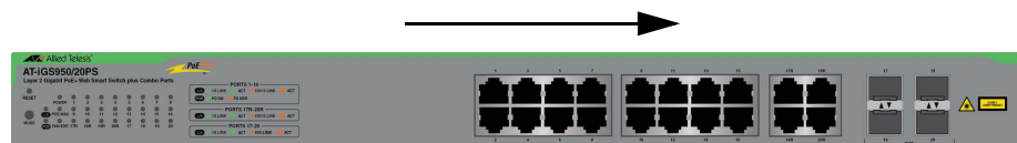
Figure 14. Ventilation Airflow of Switches with Fans
