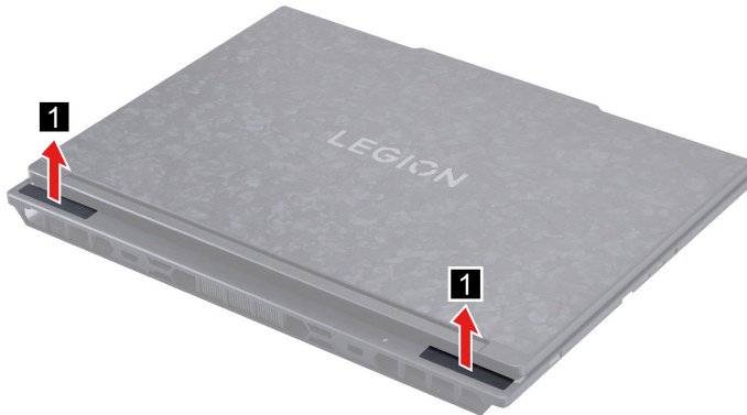
Figure 6. Remove the hinge sup mylar
