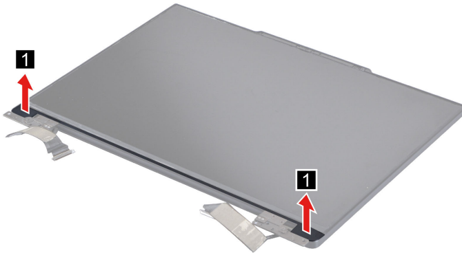
Figure 42. Remove the hinge cover
