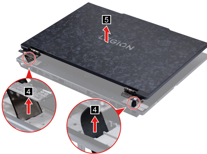
Figure 40. Remove the display assembly
