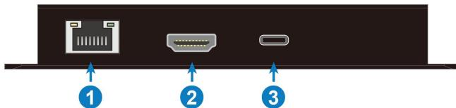
① **ETHERNET:** 1x RJ45 port, connect to Ethernet.
