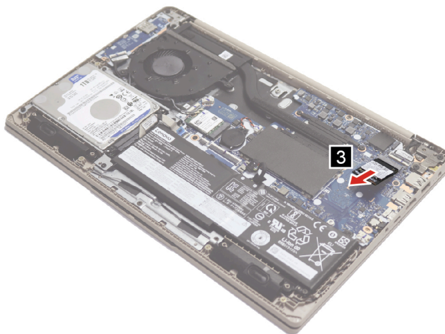
Figure 19. Remove the solid-state drive
