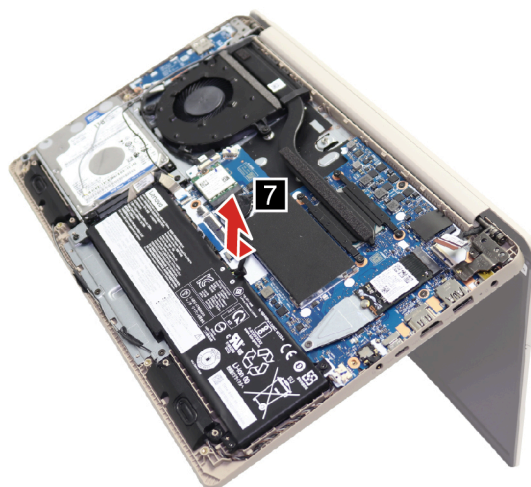
Figure 57. Remove the upper case assembly
