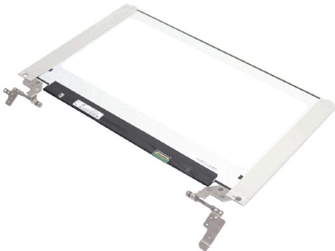
Figure 68. Remove the LCD assembly
