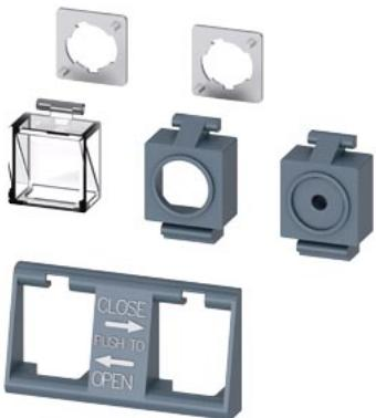
Accessory Circuit breaker 3WA, Interlocking for mechanical Open/Close without lock Set each consisting of 2 transparent covers for sealing or for attaching padlocks + cover with 6.35 mm hole + lock mount for safety lock for key operation (without safety lock)
