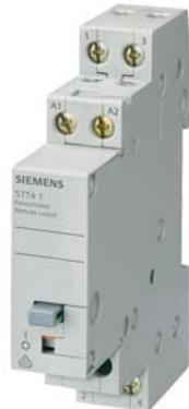
Remote control switch with 2 NO contacts, Contact for 230 V AC, 400V 16A
