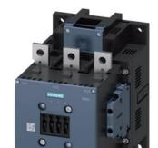
power contactor, AC-3e/AC-3 265 A, 132 kW / 400 V AC (50-60 Hz) / DC Uc: 23-26 V 3-pole, auxiliary contacts 2 NO + 2 NC permanently mounted drive: conventional main circuit: busbar control and auxiliary circuit: screw terminal
