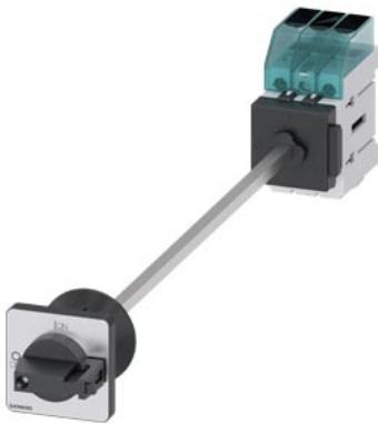
Load disconnector 3LD3, Iu 25 A Main switch 3-pole Rated operating capacity at AC-23 A at 400V 9.0kW floor mounting Basic switch with door coupling Central hole mounting 22.5mm Toggle drive black 48x48 mm
