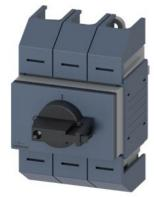
Switch disconnector 125A, size 02, 3-pole Front operating mechanism center Complete unit with direct operating mechanism gray Box terminal
