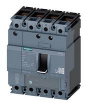
circuit breaker 3VA1 IEC frame 160 breaking capacity class N Icu=25kA @ 415V 4-pole, line protection TM220, ATFM, In=100A overload protection Ir=70A...100A short-circuit protection Ii=10 x In N conductor unprotected nut keeper kit
