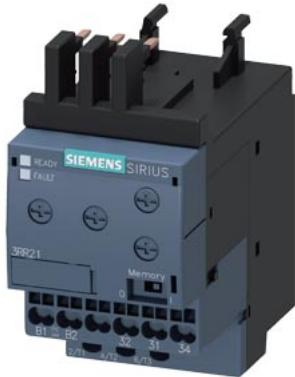
Monitoring relay, can be mounted to Contactor 3RT2, Size S00 basic, analog adjustment Apparent current monitoring 1.6-16 A, 20-400 Hz, 2-phase Supply 24 V AC/DC 1 change-over contact Monitoring for Current overshoot and undershoot Phase failure, Cable break with or without fault buffer ON delay 0-60 s Noise pulse suppression 0-30 s Switching hysteresis 6% spring-type connection system
