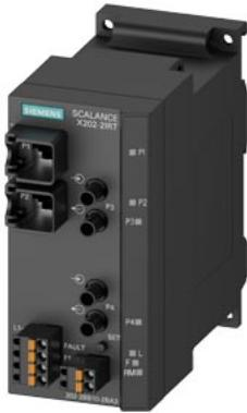
SCALANCE X202-2IRT managed IE IRT switch, 2x 10/100 Mbps RJ45 ports, 2x 100 Mbps multimode BFOC, error signaling contact with set pushbutton, redundant power supply, PROFINET IO device, network management, Redundancy Manager integrated, incl. electron. manual on CD-ROM, C-PLUG optional
