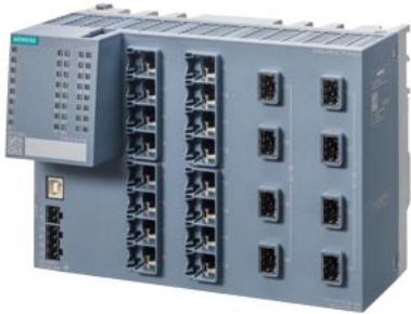
SCALANCE XCM324 managed layer 2 IE switch, 16x 10/100/1000 Mbit/s RJ45, 8x 1/10 Gbit/s SFP+ port, LED diagnostics, error signaling contact with select/set pushbutton, PROFINET IO device, network management, redundancy functions, office features (RSTP, VLAN, IGMP,..) CLP included in scope of supply assembly: DIN rail/S7 mounting rail .
