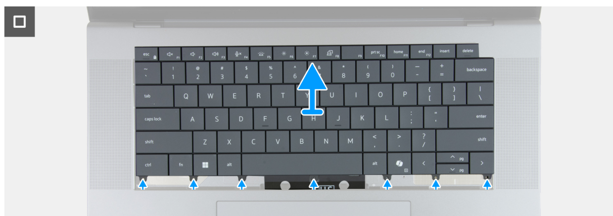
Figure 77. Removing the keyboard
