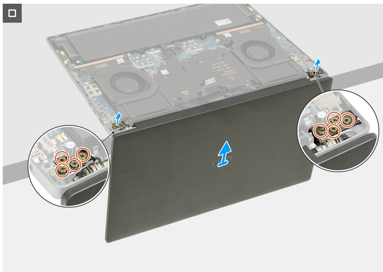
Figure 35. Removing the display assembly
