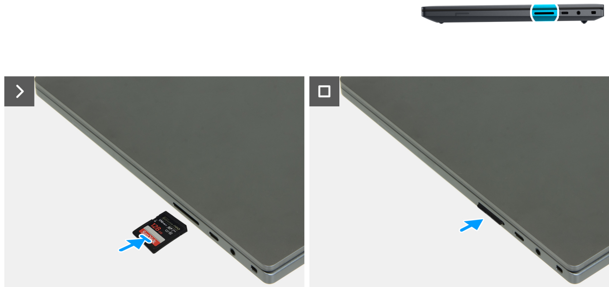
Figure 12. Installing the memory card
