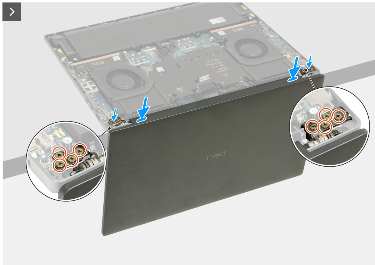
Figure 42. Installing the display assembly
