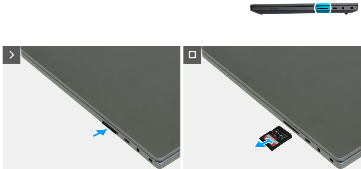
Figure 11. Removing the memory card
