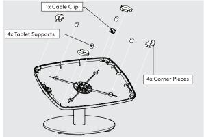
Install the Tablet Setup Kit. Each kit is specific per Tablet & Case.
