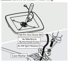
Locate and attach the Case to the Twist as shown.
