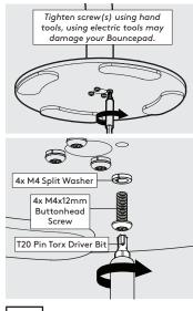
1 Locate & secure the Twist to the Counter Base.
