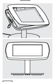
9 Locate & lock the Faceplate onto the Case.
