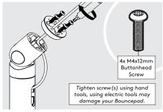
Peed Cable through Neck-Ring & cable channel. Use 4x M4x12mm Buttonhead Screws to attach Neck-Ring.
