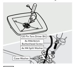
Locate and attach the Case to the Twist-Mini as shown.
