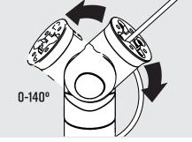
Feed Cable through channel. Test rotate & tilt to ensure enough cable slack through the full range of tilt.
