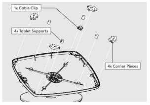
Install the Tablet Setup Kit. Each kit is specific per Tablet & Case.
