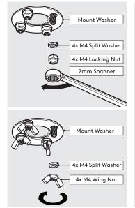
A4 Secure the Twist to the surface. Locking Nuts offer higher security.
