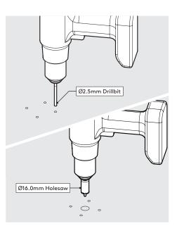
B2 Drill each hole - using the specified drill sizes.
