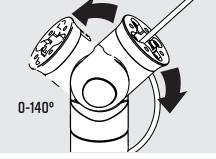
Feed Cable through channel. Test 2 rotate & tilt to ensure enough cable slack through the full range of tilt.
