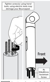
Locate and screw the Socket Screws into the Twist as shown.
