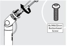
Feed Cable through Neck-Ring & cable channel. Use 4 x M4x12mm Buttonhead Screws to attach Neck-Ring.
