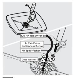
Locate and attach the Case to the Twist as shown.
