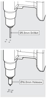
A2 Drill each hole - using the specified drill size.
