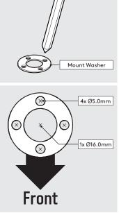
Using the Mount Washer, mark the drill hole locations as shown.
