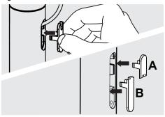
Fit cable all Cable Covers. Fit cover 'B' before cover 'A'.
