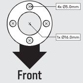
Using the Mount Washer, **A1** mark the drill hole locations as shown.
