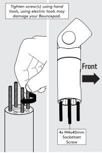
Locate & screw the Socket Screws into the Twist-Mini as shown.
