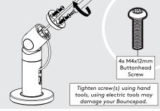
Feed Cable through Neck-Ring & cable channel. Use 4x M4x12mm Buttonhead Screws to attach Neck-Ring.
