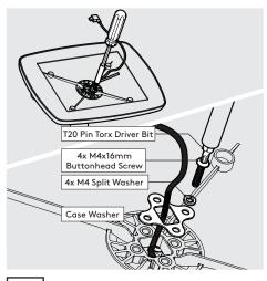
4 Locate & attach the Case to the Twist-Mini as shown.
