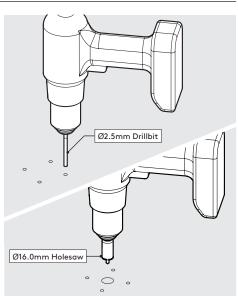
Drill each hole - using the specified **B2** drill sizes.
