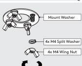
Secure the Twist-Mini to the surface. Locking Nuts offer higher security.
