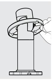
B3 Locate the Cover onto the Twist-Mini.
