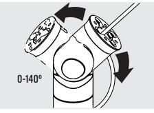
Peed Cable through channel. Test rotate & tilt to ensure enough cable slack through the full range of tilt.
