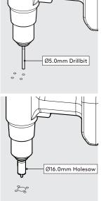
Drill each hole -**A2** using the specified drill size.
