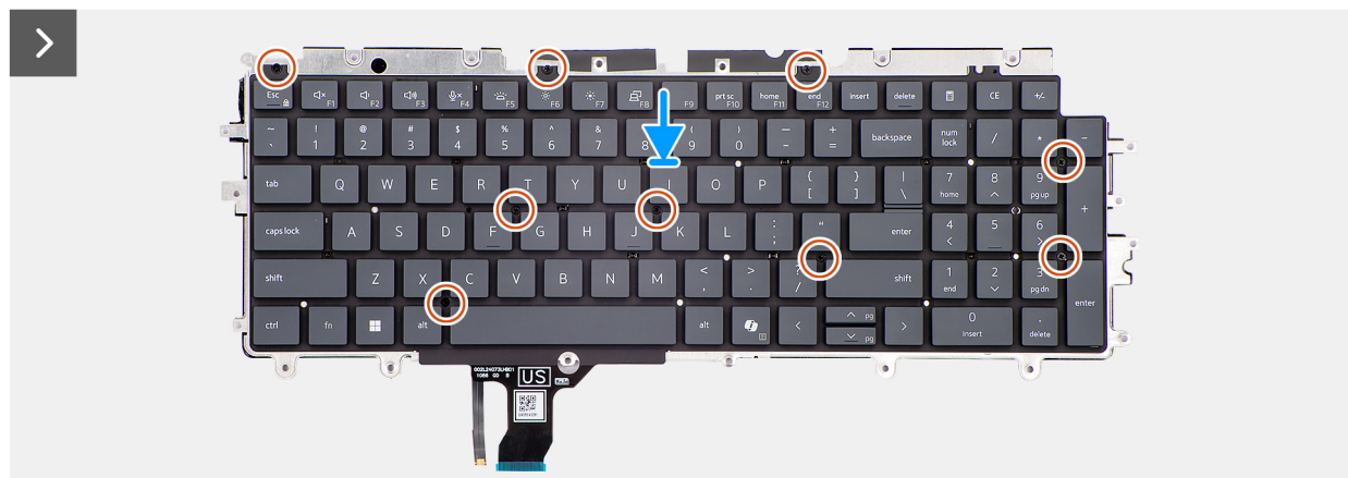
Figure 100. Installation du clavier
