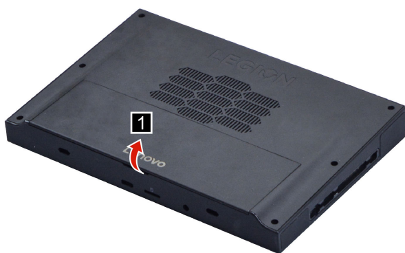
Figure 9. Open the stand cover to maximum angle
