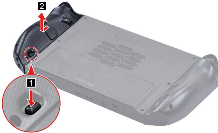
Figure 6. Remove the Legion Go 2 Controller R
