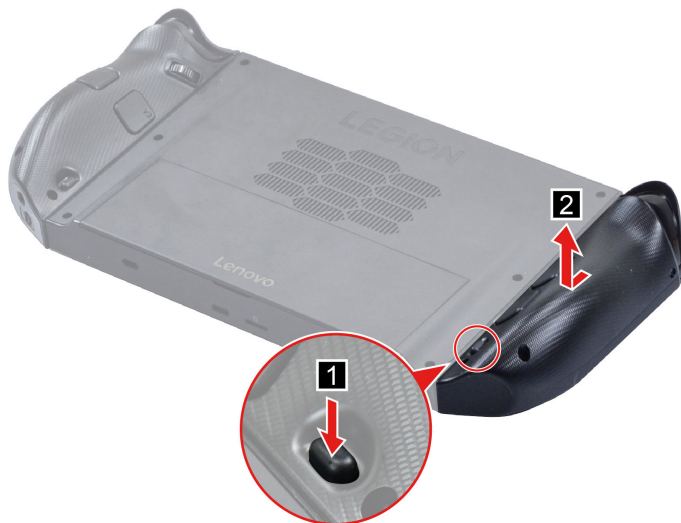
Figure 5. Remove the Legion Go 2 Controller L
