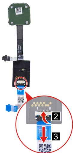
Figure 26. Remove the fingerprint board FFC
