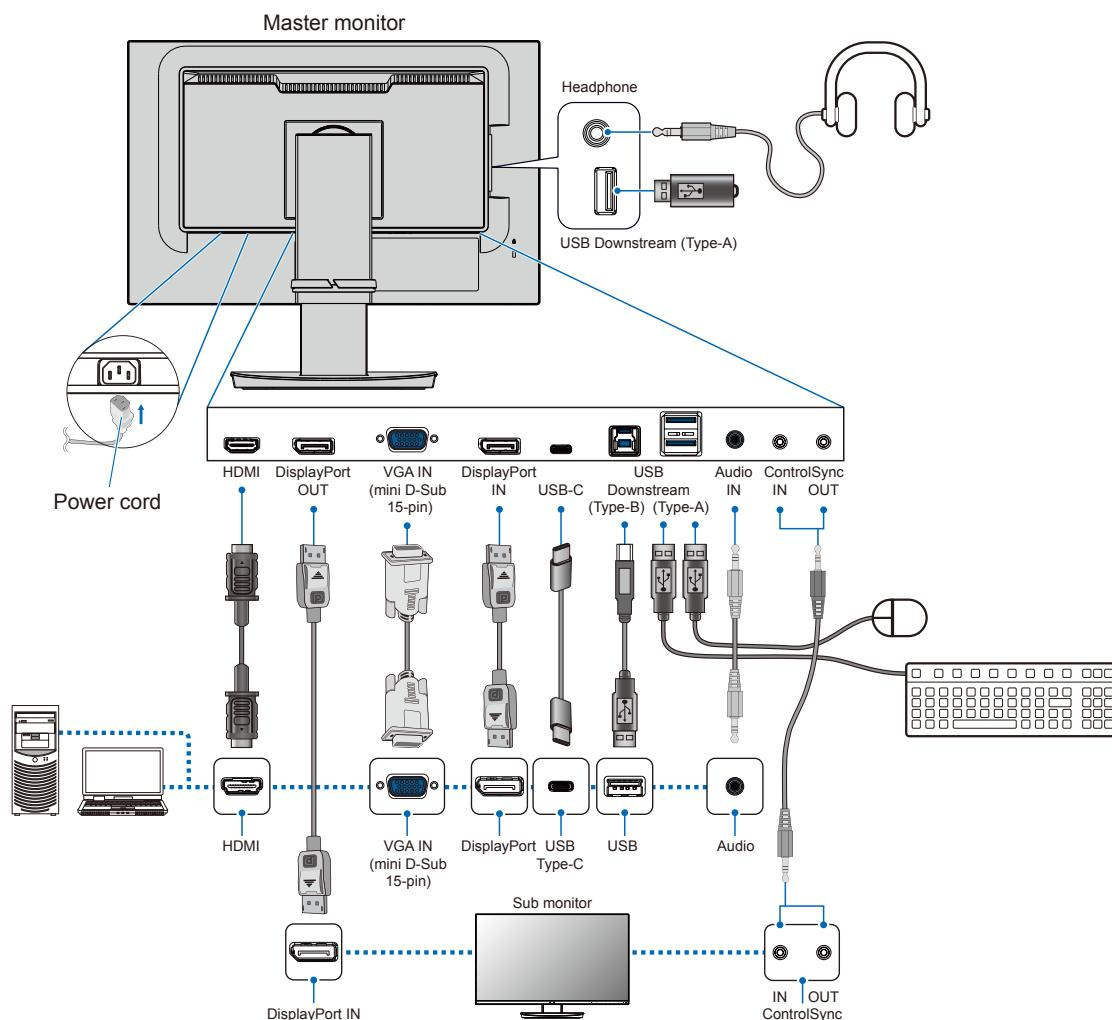
To maintain compliance with EMC regulations, use shielded cables to connect to the following terminals: HDMI IN, DisplayPort IN, USB Downstream Port (Type-A), USB Upstream Port (Type-B) and USB-C port. Use shielded signal cables with ferrite core to connect to the following terminals: VGA IN.
