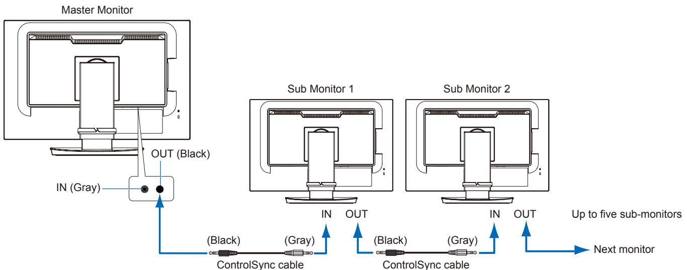
**TIP:** The ControlSync icon will appear on the upper left of the OSD menu in the sub-monitors. Do not connect the ControlSync ports IN-to-IN or OUT-to-OUT. The monitors' ControlSync ports must be connected OUT-to-IN.
