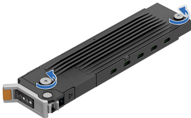
Figure 174. Loosen the top cover captive screws
