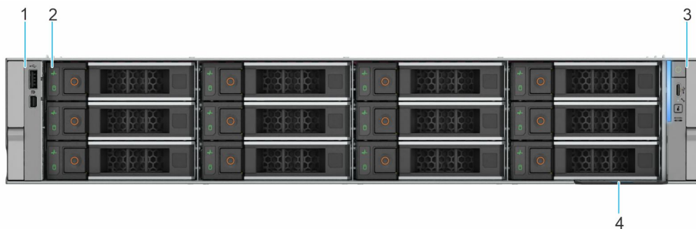
Figure 3. Front view of the 12 x 3.5-inch SATA/SAS
