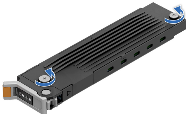
Figure 183. Loosen the top cover captive screws
