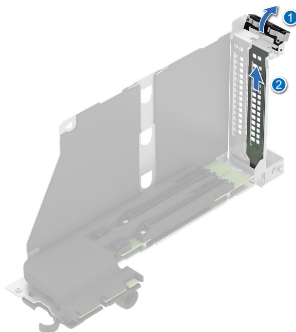
Figure 170. Removing the filler bracket
