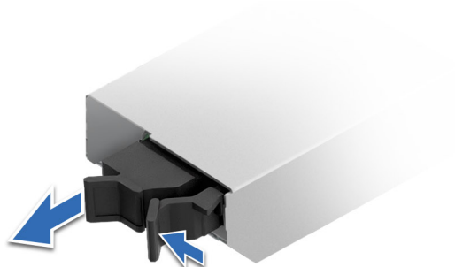
Figure 214. Removing the BOSS-N1 DC-MHS card carrier blank
