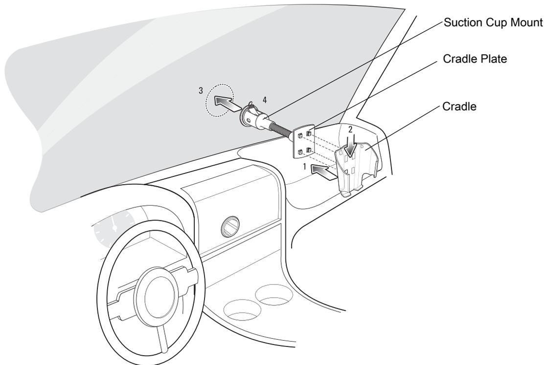
2. Flip the lever down to create a vacuum between the suction cup and the mounting surface.
