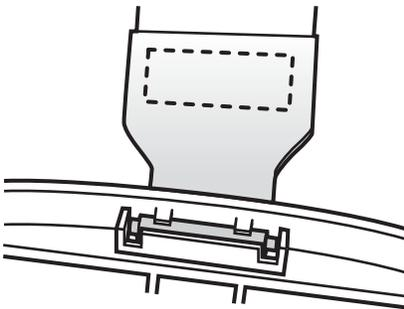
**Figure 43** Slide Handstrap and Tether Over Handstrap Mount
