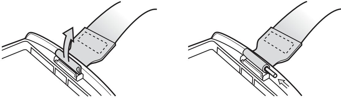
2. Slide pin into bottom of handstrap.
