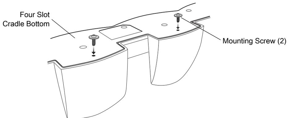
2. Align the Wall Mount Bracket mounting tabs with the mounting slots in the back of the four slot cradle. Slip the two mounting tabs into mounting slots.
