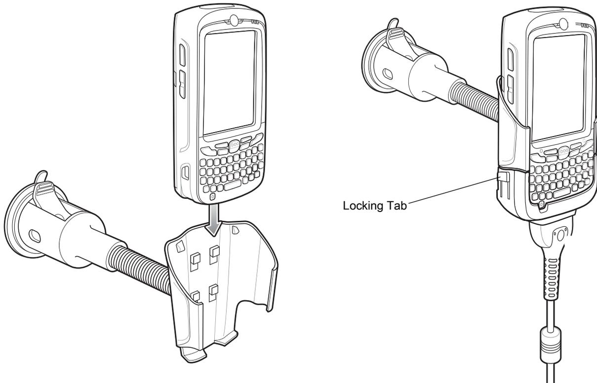
5. Connect the auto charger cable to the MC55X and slide the two locking tabs up to secure the cable cup to the MC55X.
