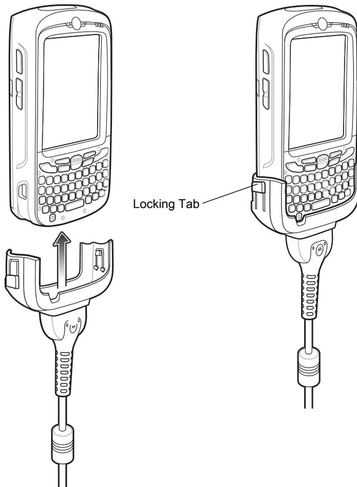
4. To remove, slide the two locking tab down and remove the cable from the MC55X.
