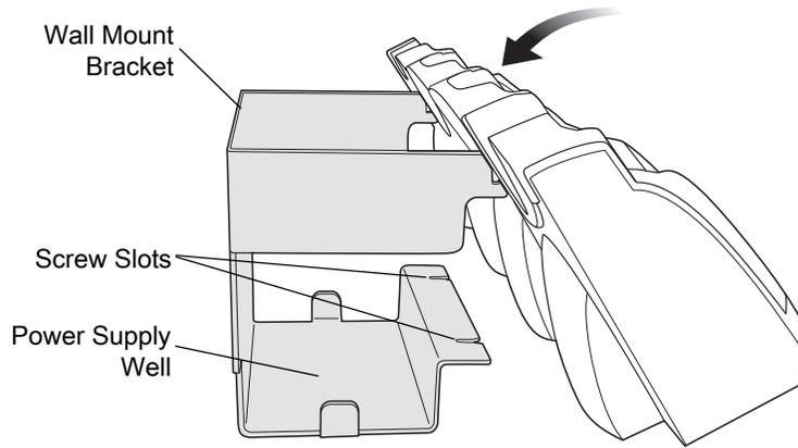
4. Tighten the mounting screws to secure the four slot cradle to the bracket.
