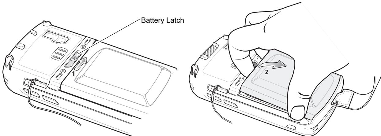
7. Lift the battery from the MC55X.
