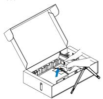
Press the button to remove the rear pillar cover
