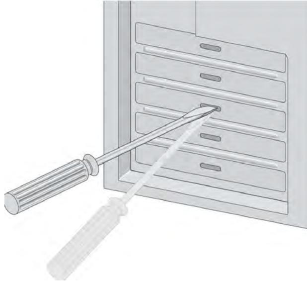
Figure 13. Removing the Faceplate From PCIe Slot
