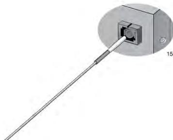
Figure 67. Cleaning a Recessed Ferrule
