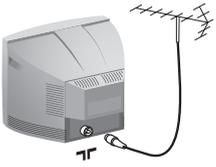
Insert the aerial plug into the
