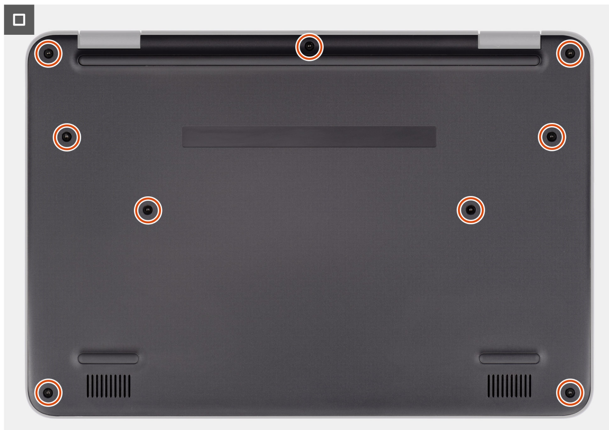
Figure 21. Installing the base cover
