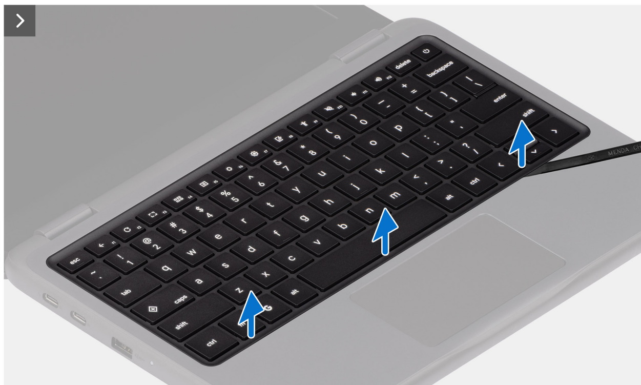
Figure 29. Releasing the keyboard with a scribe
