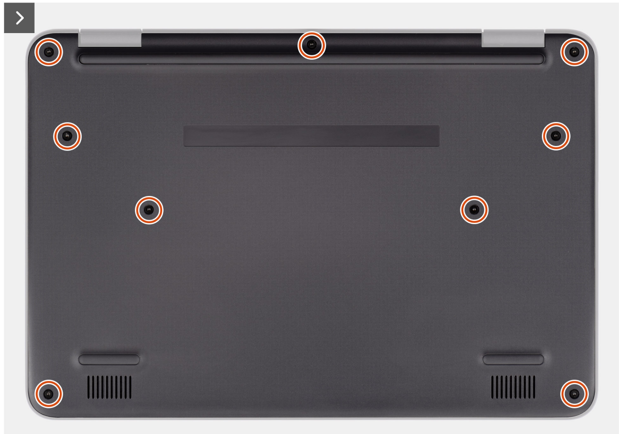
Figure 18. Removing the base cover
