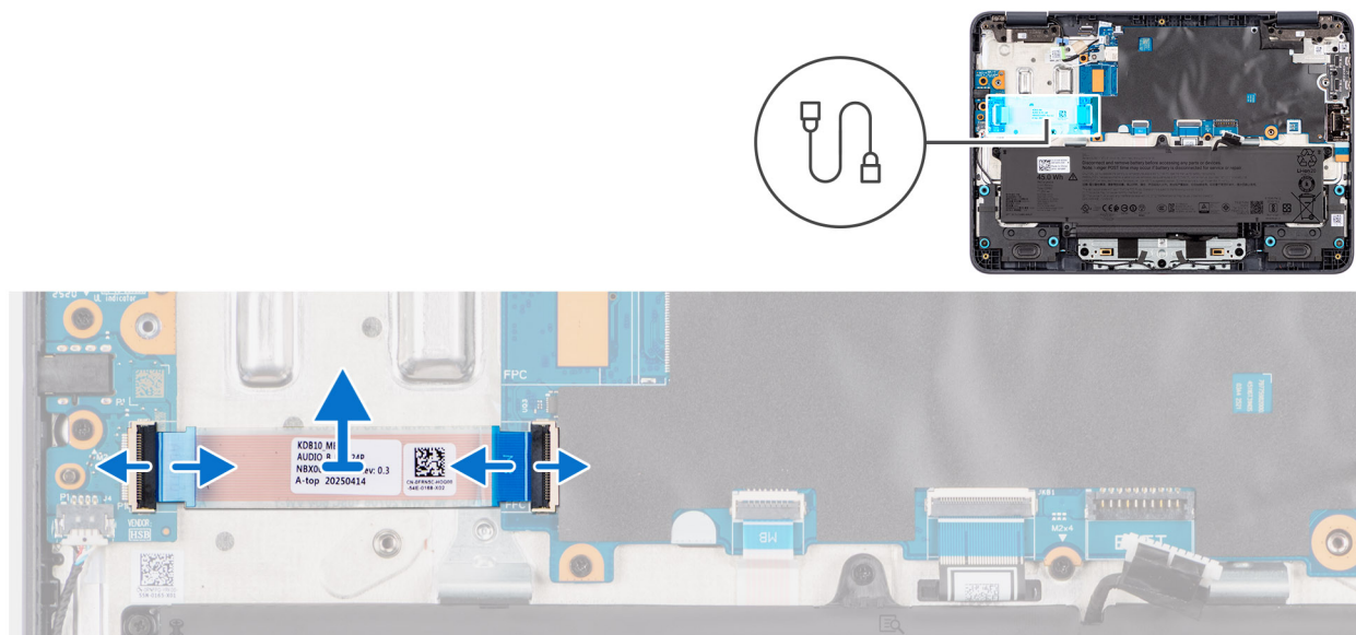
Figure 12. Removing the I/O board cable
