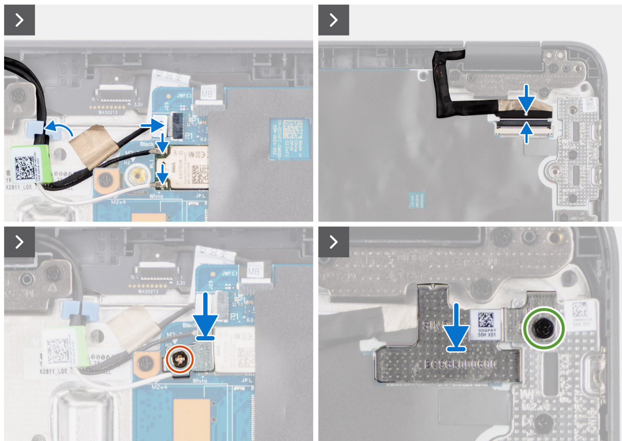
Figure 59. Installing the display assembly
