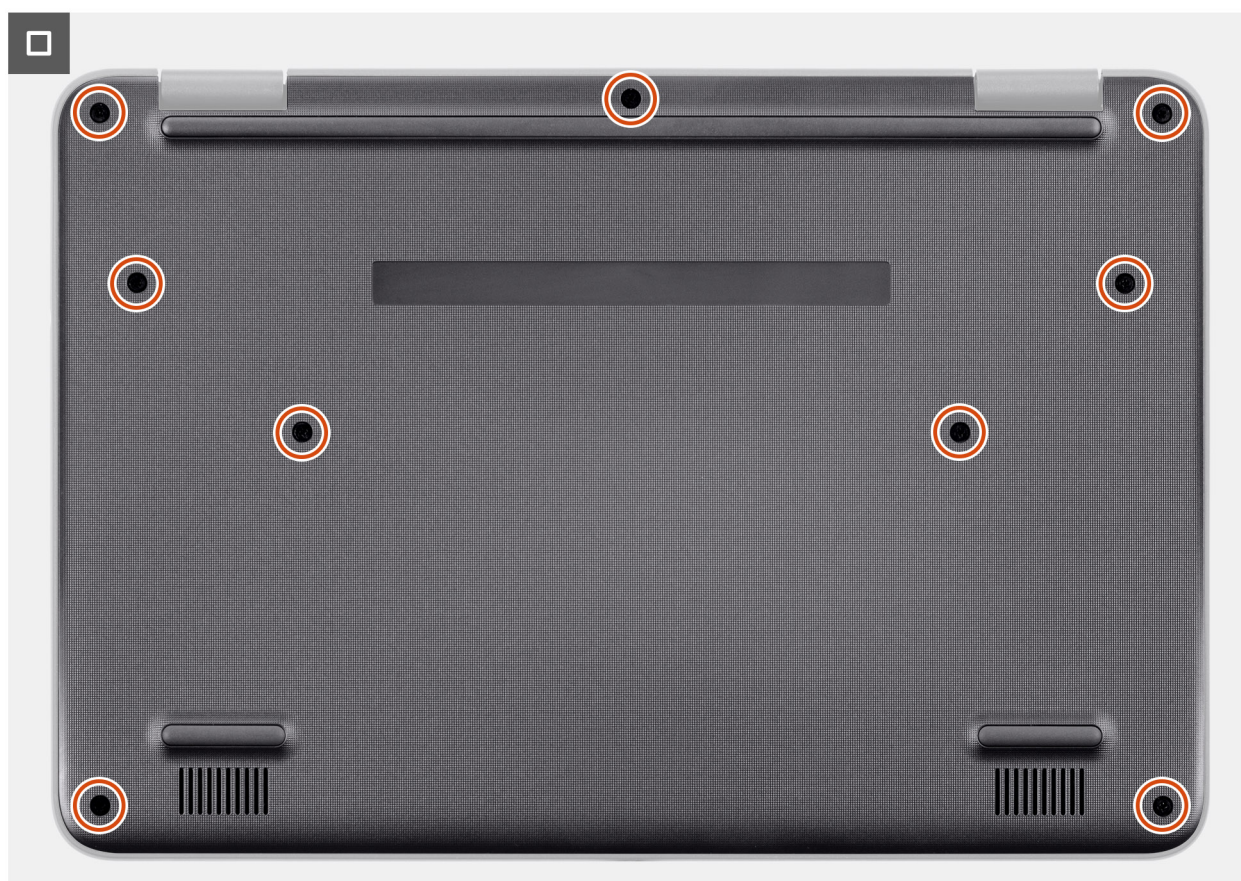
Figure 7. Tightening the base cover screws
