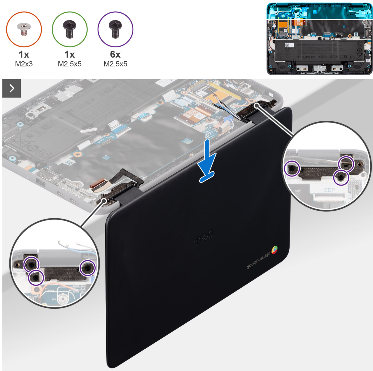
Figure 57. Installing the display assembly
