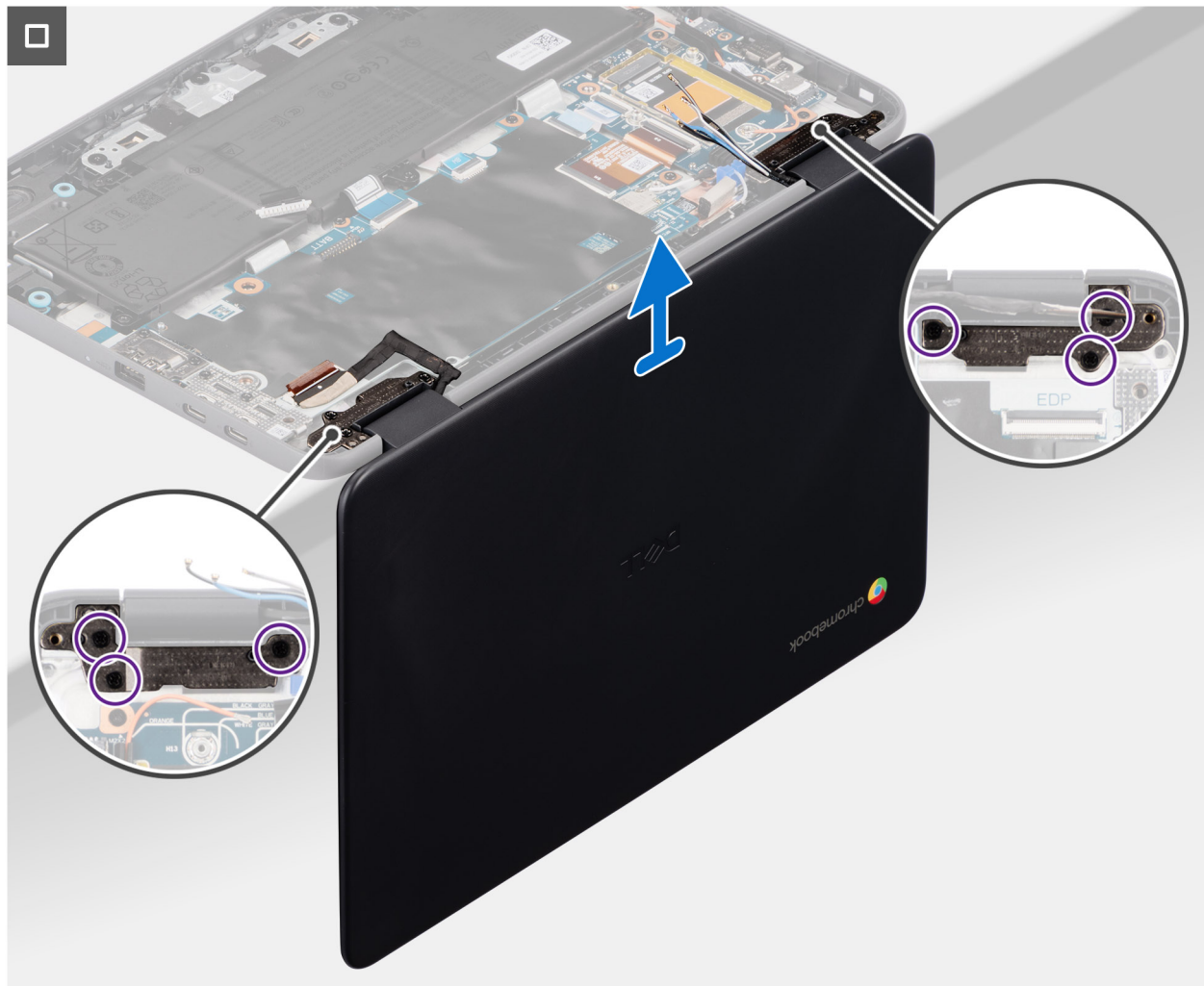
Figure 55. Removing the display assembly
