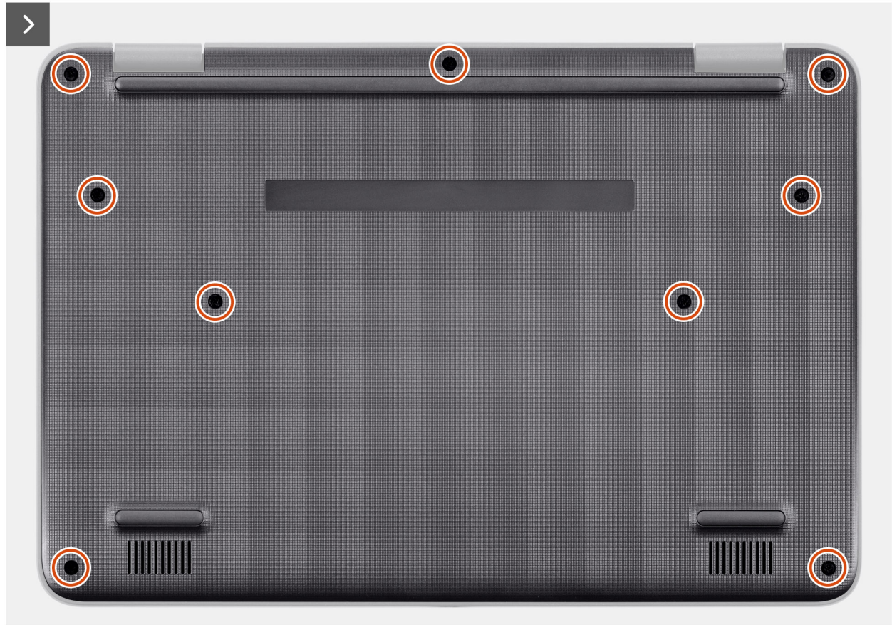
Figure 2. Loosening the base cover screws
