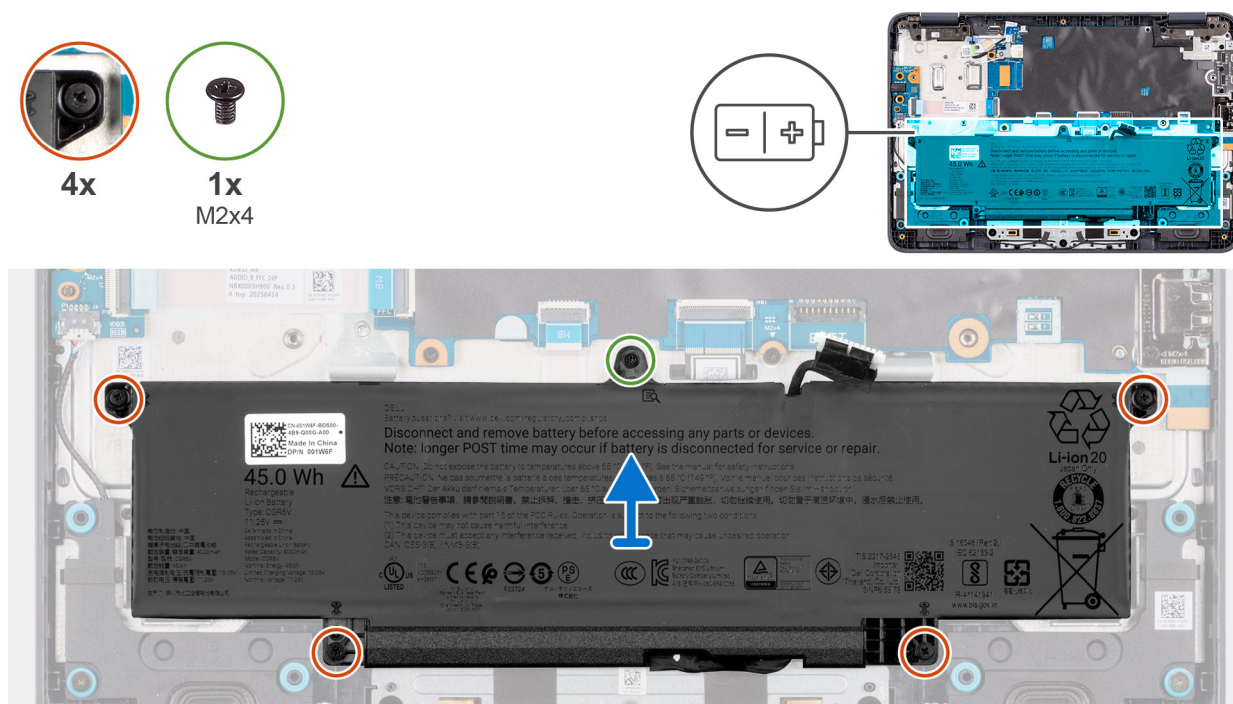
Figure 8. Removing the battery
