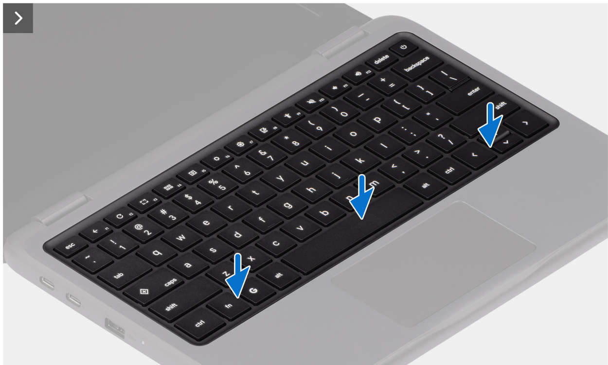
Figure 32. Installing the keyboard
