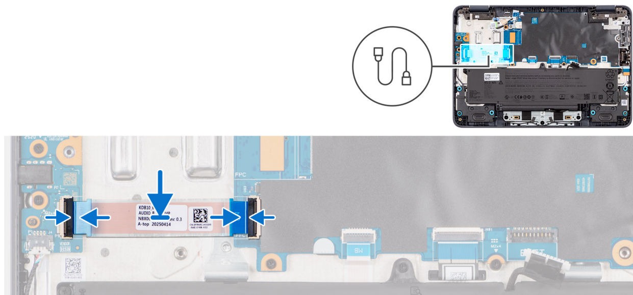
Figure 13. Installing the I/O board cable
