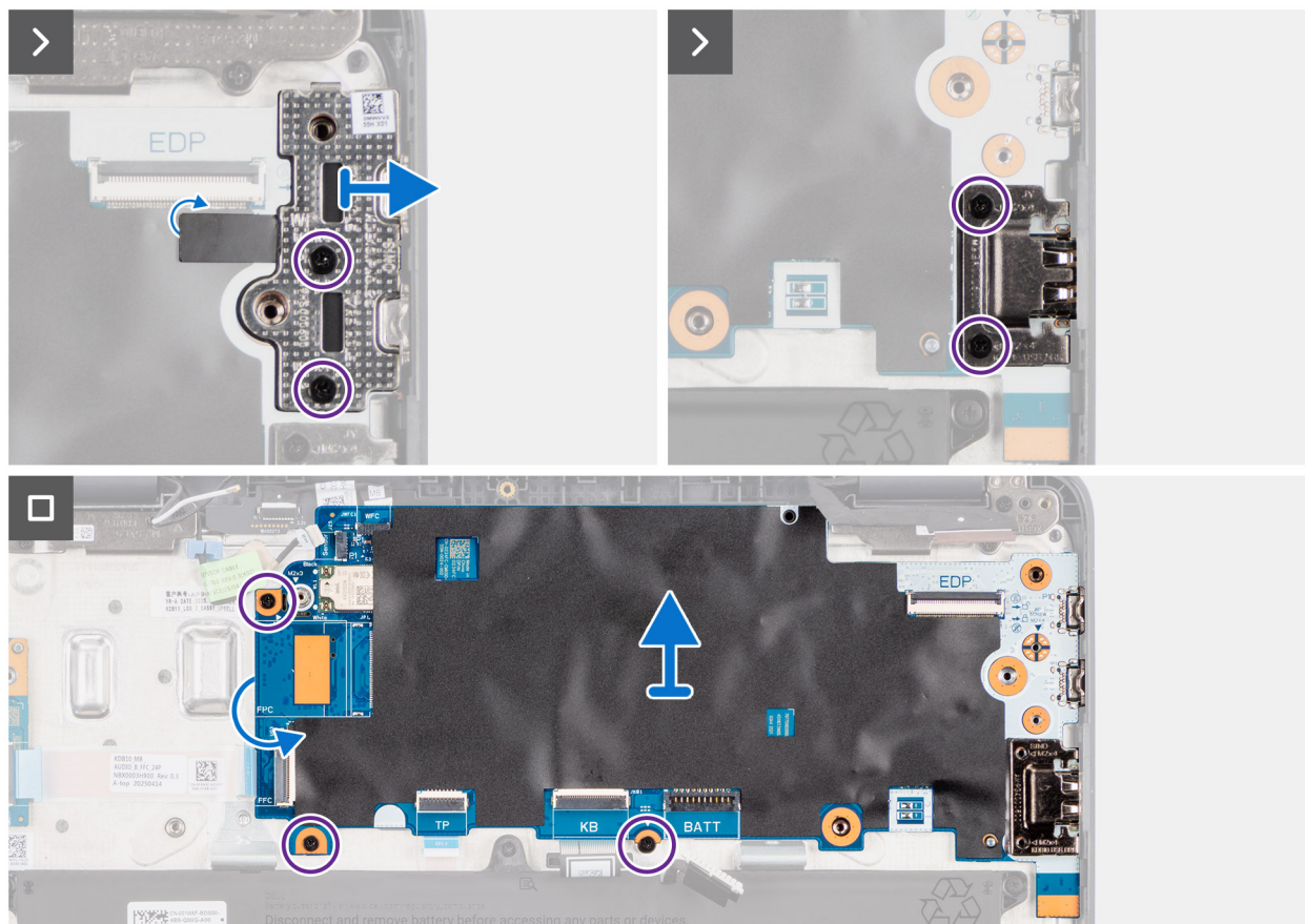
Figure 28. Removing the system board
