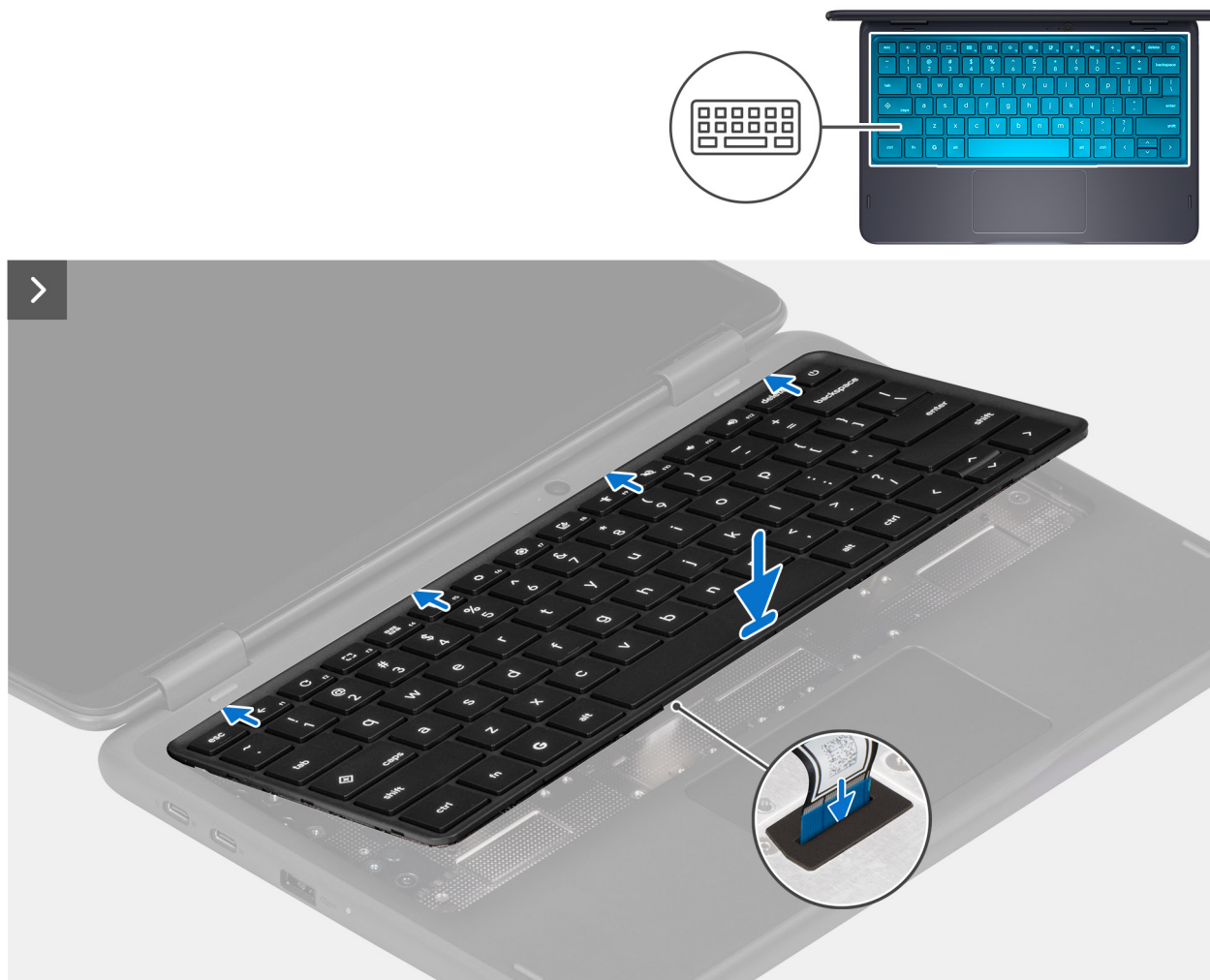
Figure 21. Inserting the keyboard cable through the opening on the palm-rest assembly and placing the keyboard on it
