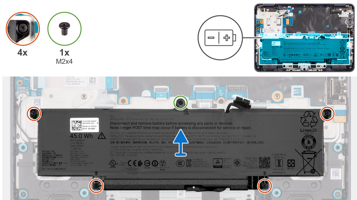
Figure 8. Removing the battery
