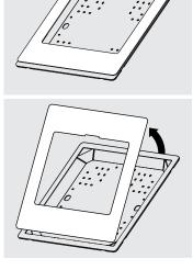
Remove the Faceplate from the Case by pushing upwards & pivoting.
