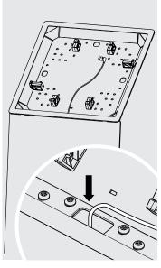
Feed the Tablet's Power Cable through the Case & Mounting Arm.
