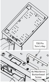
Attach the Case to the Mounting Arm & Printer Mount. Ensure the Case is aligned.
