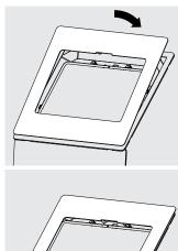
Locate the Faceplate to the Case by pivoting & pushing downwards.
