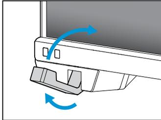
2. When the color sensor reaches the edge of the screen, it will stop and start the calibration process. The calibration time depends on the amount of preset modes you select, the longest time might be 30 minutes.
