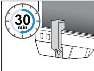
3. After the calibration process is completed, the color sensor will automatically return to its original position.
