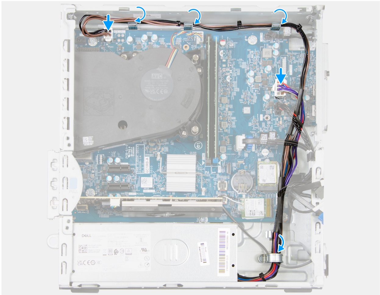
Figure 51. Installing the power-supply unit
