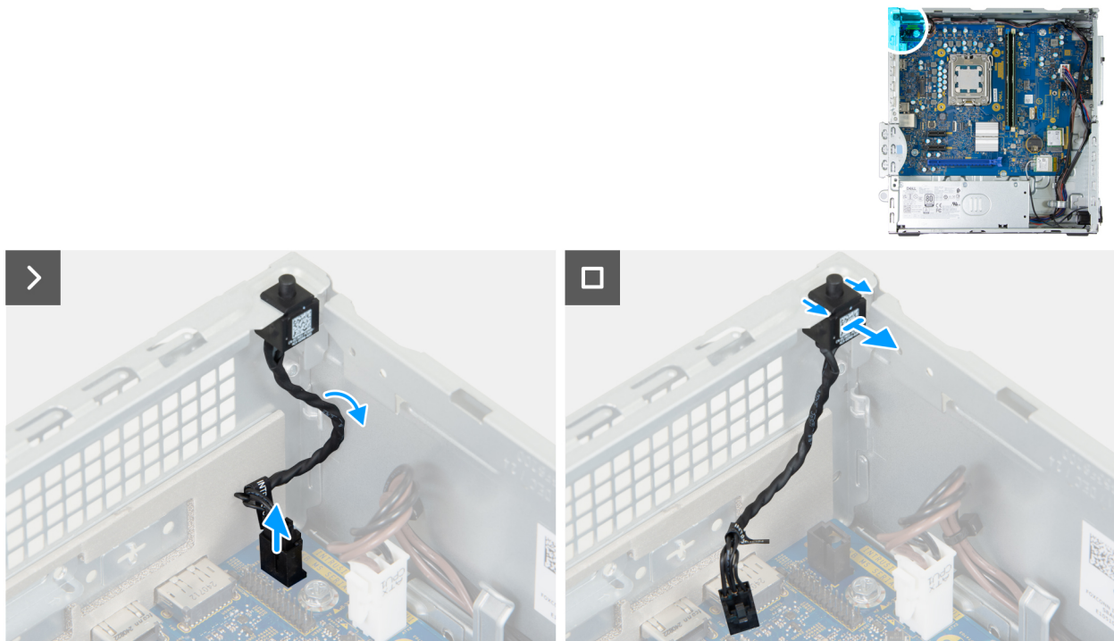
Figure 42. Removing the intrusion switch
