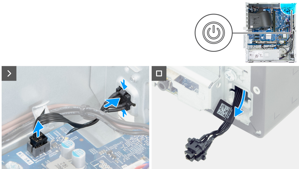
Figure 51. Removing the power button
