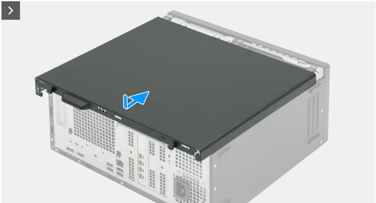
Figure 15. Installing the left-side cover
