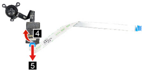
Figure 24. Remove the fingerprint board cable
